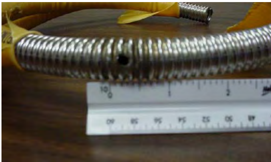
Example of Damage to CSST
